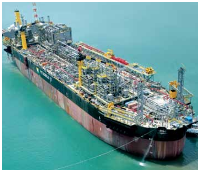
After a successful preconversion at Keppel Shipyard in Singapore, FPSO P-57 will have her newly fabricated topsides installed and integrated at Keppel's BrasFELS yard.
