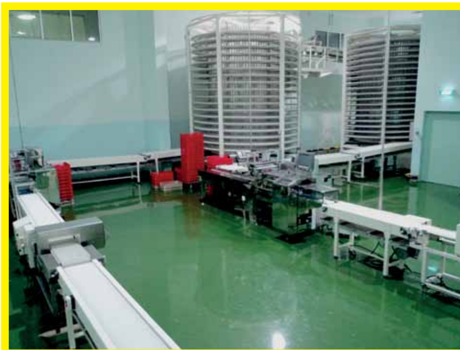
Spiral Conveying System Available for : Cooling - Freezing - Fermentation - Steaming - Aging Process - Oven / Baked. Suitable for Bakery, Ice Cream, Meat, Seafood, etc.
