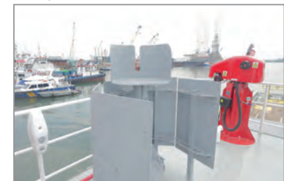
Gun mount with ballistic shields and fire fighting monitor.
